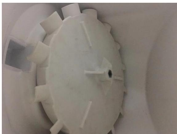
4. Slide the paddle wheel from the motor shaft and remove.
