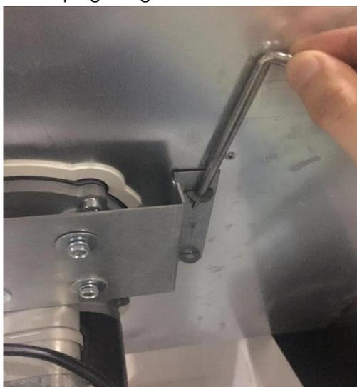
4. Pull the disassembly pin up.
