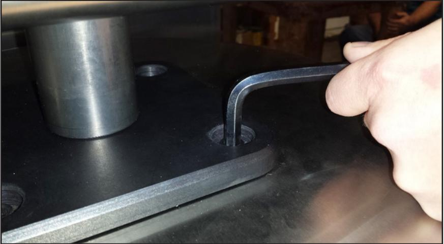
4. Adjust the front height of the upper platen up by turning the adjustment nut counter clockwise. Turning the adjustment nut clockwise will lower the front of the platen. Adjust in 180 degree increments, alternating between the two nuts being adjusted.
