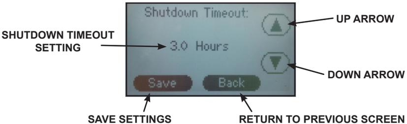
2. Press the “UP” ▲ and/or “DOWN” ▼ arrows to set the desired shutdown time.
