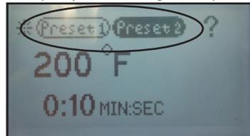
1. Press and release for approximately 1/2 second the preset button to recall. The controller will beep and the preset location button will display in reverse indicating the preset has been changed.
