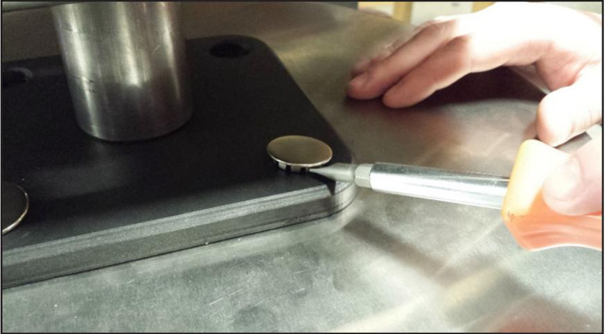
2. Lower the Top Platen until one side touches to determine which side will be adjusted. In the picture below, the front of the platen could be raised or the back could be lowered.
